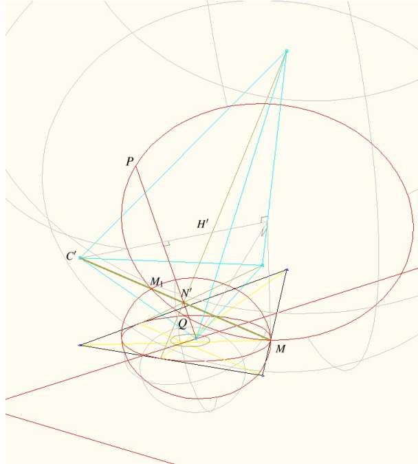
Figure 7: C'M is the radical axis of the two circles of intersection
